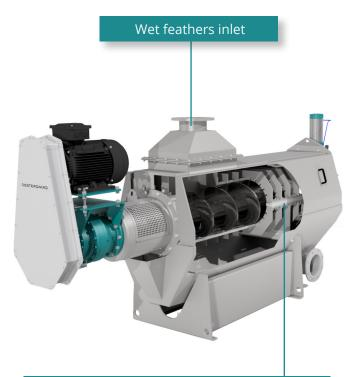
Water is squeezed out of the feathers and drained through the perforations in the strainer plates
